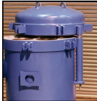
Left: Handle Davit headlift on a FW micronic filter vessel
